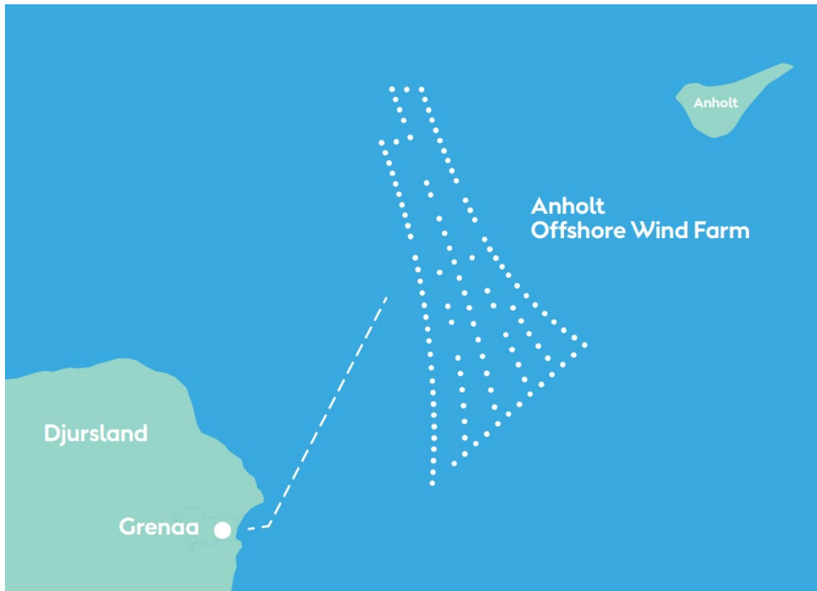
Figure 8.B. The Anholt Offshore Wind Farm. White dots = 111 wind turbines. Dotted line = undersea cable. (Source: https://orsted.com/-/media/www/docs/corp/com/our-business/wind-power/wind-farm-project-summary/anholt_uk_2018.ashx?la=en&hash=7707175e111c65a4aefc353291091ee4 )
