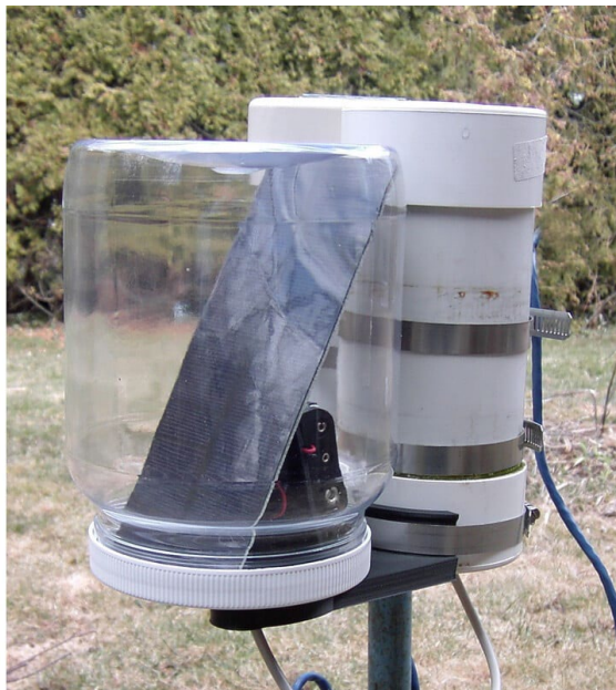
Figure 6.4.A Equipment for Anholt 2, the new, second fixed measuring station on Anholt: a Unihedron Photometer SQM sky quality meter with lens, waterproof housing for Sky Quality meter, and Solar Charger.
